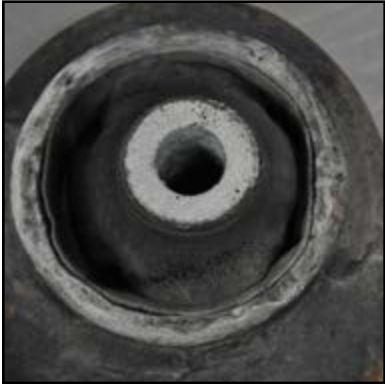
Control arm bushings collapsed off center and separating from the outer cage
