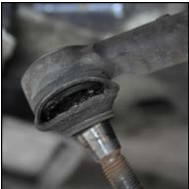
Torn tie rod and ball joint boots
