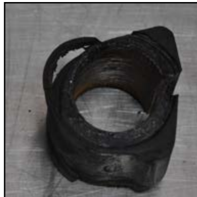
Worn out, torn sway bar bushings
