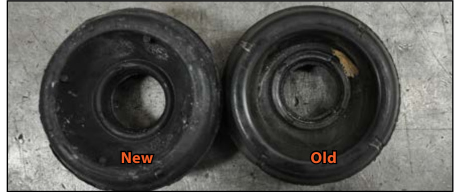
Upper strut mounts worn off center
