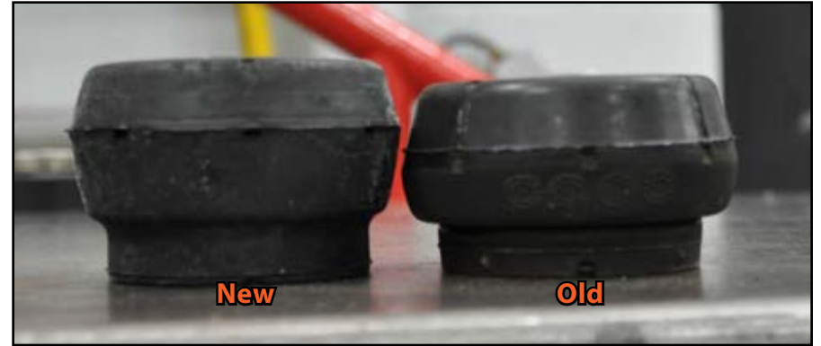
Collapsed upper strut mounts
