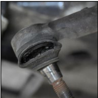
Torn tie rod and ball joint boots
