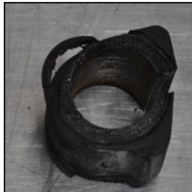
Worn out, torn sway bar bushings
