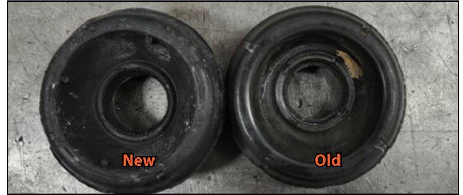
Upper strut mounts worn off center
