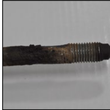
Rusted away and weakened bolts and fasteners
