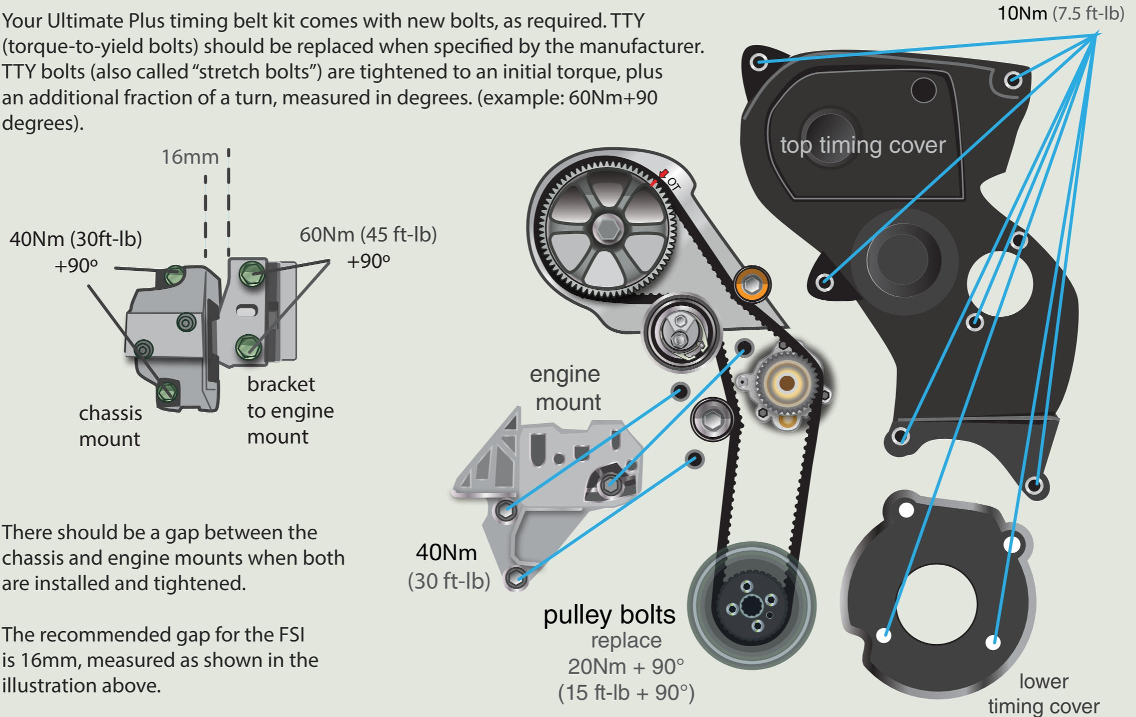
There should be a gap between the chassis and engine mounts when both are installed and tightened.
