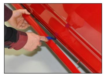
Work your way down the side, using heat as required, and pulling the side blade off the body studs as you go.
