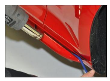
Start at either end and carefully use a heat gun to release the adhesive tape and a non marring trim tool to lift the side blade from the body.
