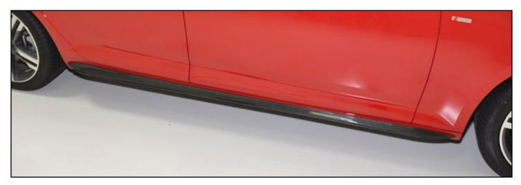
Pull the protective strip off the adhesive tape, align the new side blade over the five studs on the body and push it into place. Hold pressure for a few seconds along the entire length of the side blade to help the tape to stick.
