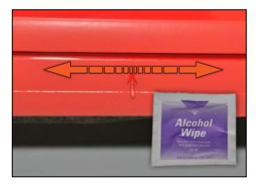
Using an alcohol pad, wipe the full length of the rocker panel along the top edge to remove any wax or oily residue.
