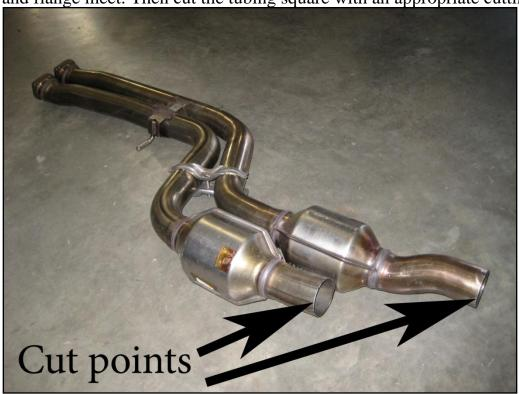
ii. Left side pipe cut point is 3 3/4" from the weld.
