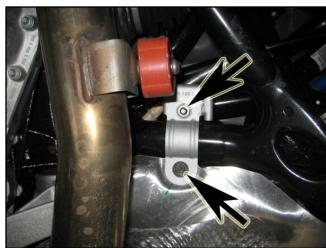
8. Unbolt the exhaust hangers at the rear bumper. Remove the two nuts on each exhaust hanger with a 13mm socket. Note the hangers stay on the exhaust.
