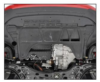
On some models (such as this MK7 GTI) the lower insulation panel does not need to be removed. Others may have a full length panel or skid plate which you will have to remove for access from underneath.
