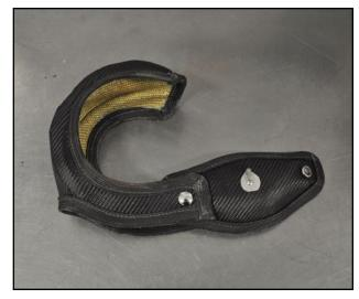
On some models, such as the Golf R, it is much easier to snap one side of the blanket together, then guide the other side through between the turbo and cylinder head.
