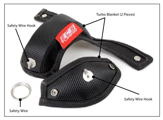
Use this photo for installation reference. It is possible that the safety wire hooks may rotate during shipment. Before you begin, be sure the safety wire hooks on your blanket are oriented as shown in this picture. Use the flat side on each hook base as an additional visual aid to orientation.
