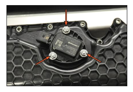
Step 12: 10mm Socket & Torque Wrench
