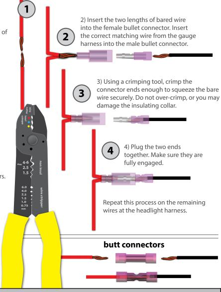
Use the same methods to splice the gauge power harness to the extension harness using butt connectors.
