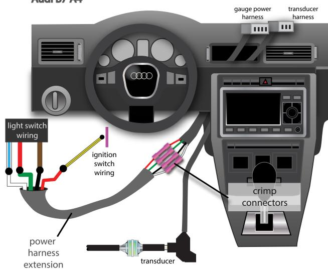
Use the length of wire in the kit with the crimp connectors to extend the length of the power harness.
