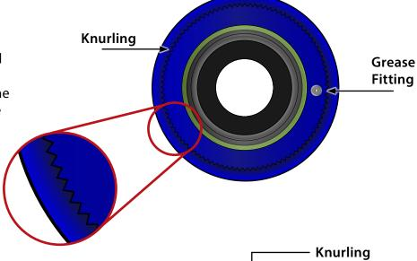
Looking at the side view, you can see the larger diameter lip on the front side, the knurling around the circumference, and the grease fitting on the rear.
