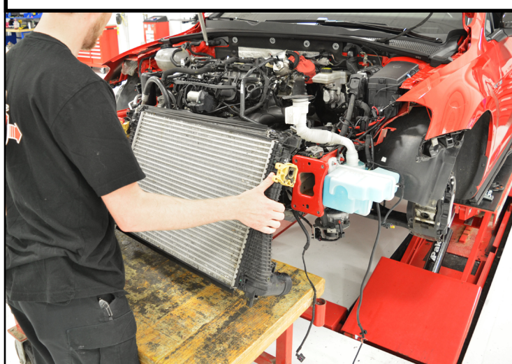
#3: Remove OE intercooler from vehicle
