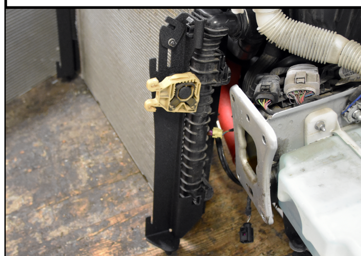
#4: Install intercooler delete brackets into vehicle
