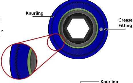
Looking at the side view, you can see the larger diameter lip on the front side, the knurling around the circumference, and the grease fitting on the rear.
