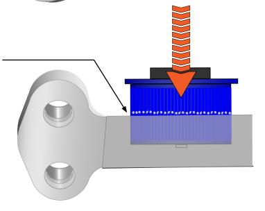
If the spherical bearing is binding after installation, press it back out, thoroughly clean all burrs from the bushing and bushing bore, then press the bushing back into place. In some cases, you may have to do this more than once, depending on variations in bracket tolerance.
