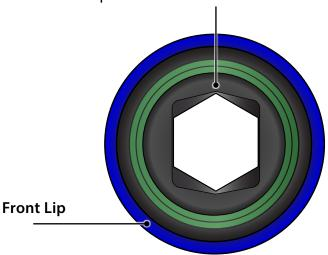
The rear of each bushing is quickly identified by the grease fitting. You will also see the knurled section around the entire circumference of the body. On the vehicle, this side will face the rear of the car.
