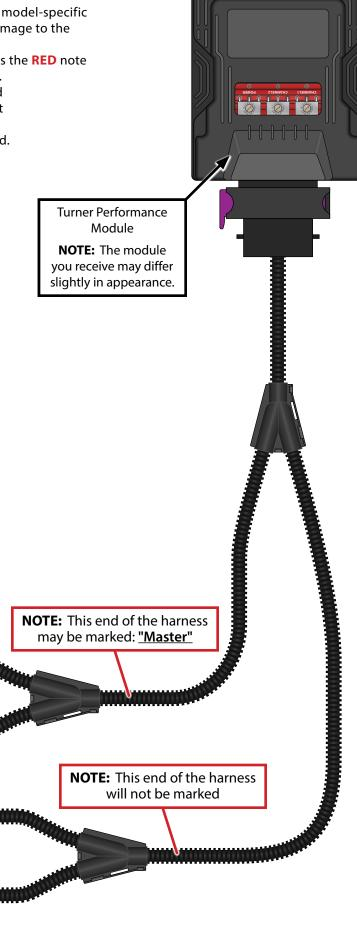
Connects to boost pressure sensor (located on the charge pipe, near the throttle body)
