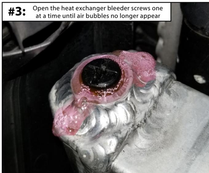
**#3:** Open the heat exchanger bleeder screws one at a time until air bubbles no longer appear
