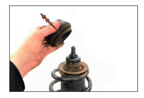
21mm Strut Nut Socket & Ratchet, 7mm Hex (Allen) Step 16:
