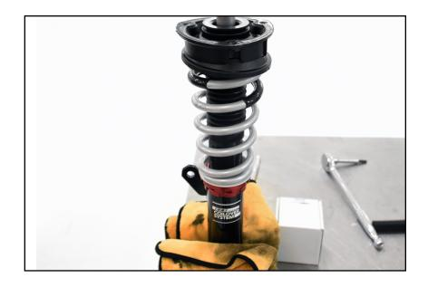
19mm Strut Nut Socket & Torque Wrench, 5mm Allen Step 2:
