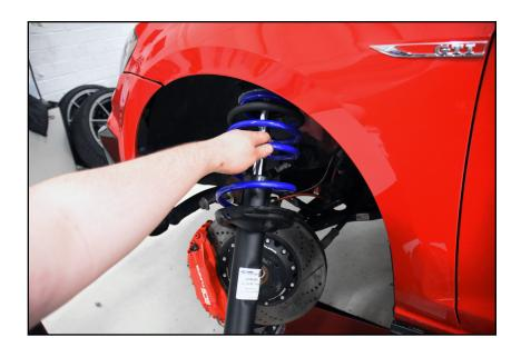
21mm Strut Nut Socket & Ratchet, 7mm Allen Step 14:
