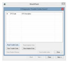
Click [Read Trouble Codes]. There may be some harmless codes here after flashing the ECU. These are typically message errors from programming.
