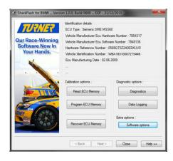
This is the main Turner Shark functions menu. At the top is the specific info for your car's ECU. At the bottom are the buttons for running the various Turner Shark functions –
