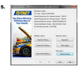
This is the main Turner Shark functions menu. At the top is the specific info for your car's ECU. At the bottom are the buttons for running the various Turner Shark functions –
