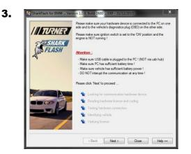
Check the condition of your car's battery. Do not continue if the battery is old, does not hold a charge, or the "**Increased battery discharge!**" warning is shown on the iDrive. Turn off all electrical loads – air conditioning, interior lights, headlights, radio, etc.
