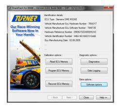
The first action is to check for existing fault codes in your ECU. This is also a communications test between your car and the Turner Shark tool.
