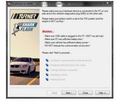
Check the condition of your car's battery. Do not continue if the battery is old, does not hold a charge, or the "Increased battery discharge!" warning is shown on the iDrive. Turn off all electrical loads – air conditioning, interior lights, headlights, radio, etc.
