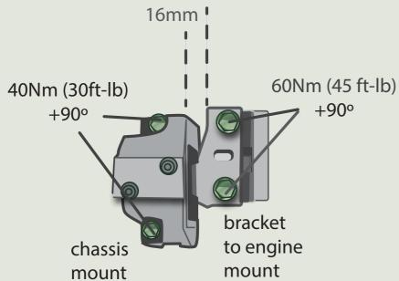
There should be a gap between the chassis and engine mounts when both are installed and tightened.
