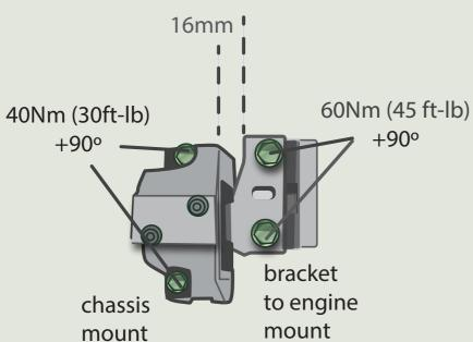
There should be a gap between the chassis and engine mounts when both are installed and tightened.
