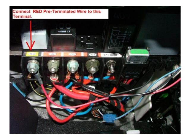
Connect the red pre-terminated wire to terminal 75x (black wires with yellow stripe) This supplies the harness with +12V
