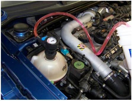
You may need to shut the engine down and repeat this process more than once to purge all air from the system. Just remember that the system will be under pressure when hot, so don't open the pressure cap to correct the coolant level until the system cools.
