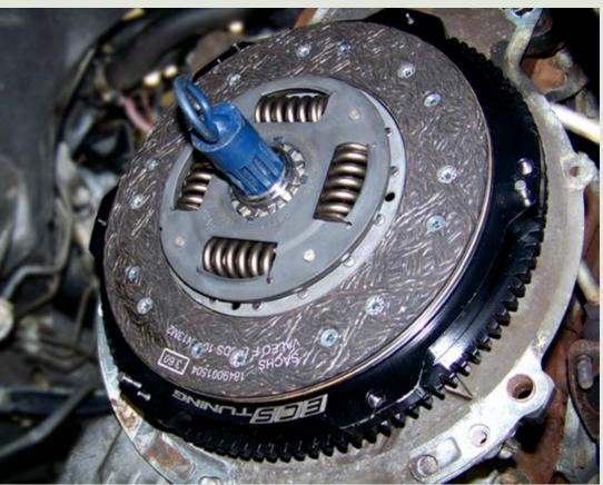
Wipe the friction face of the clutch pressure plate with a clean cloth, moistened with brake cleaner (NOT carb cleaner) to remove any oil residue.
