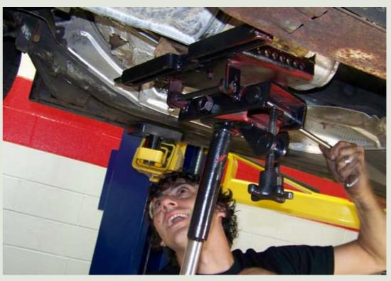
Unbolt the six hex-head pressure plate bolts and remove the pressure plate and clutch friction disc.
