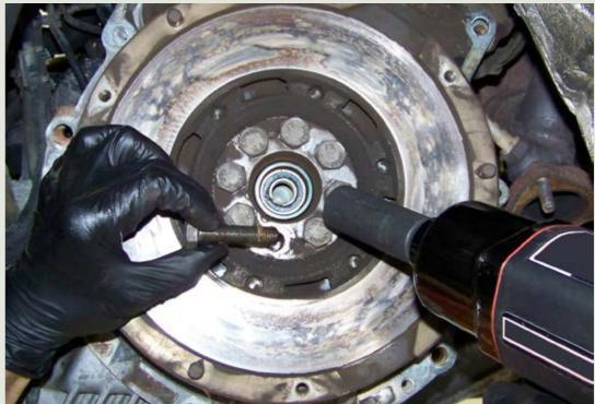
Replace the pilot bearing. The old bearing may pull out easily by hand, although some (like this one!) will stick. A puller with expandable jaws and slide hammer removes it quickly.
