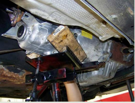
Use the two raised dowels on either side of the engine to align the transmission and engine; that's what they're there for!
