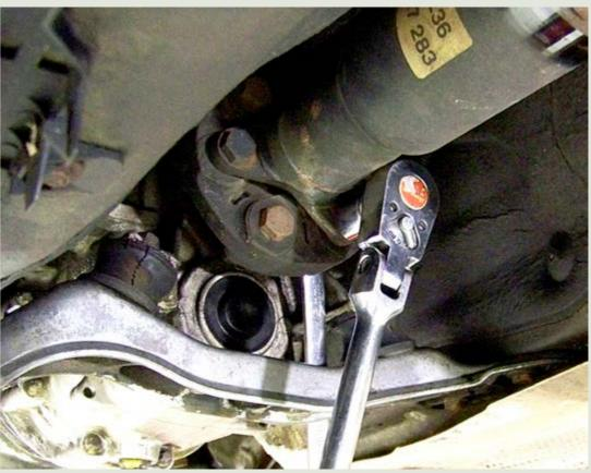
The driveshaft is a two-piece design with center universal joint, supported in the middle by a center bearing mount, bolted to the chassis by a support bar.
