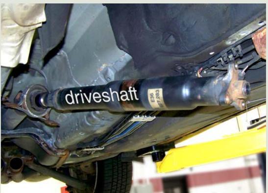
Stop here and inspect the flex coupler and center support for signs of wear or damage. Make sure the center support bearing spins freely on the driveshaft, without noise or sticking. Check the rubber donut surrounding the bearing for tears or cracks.
