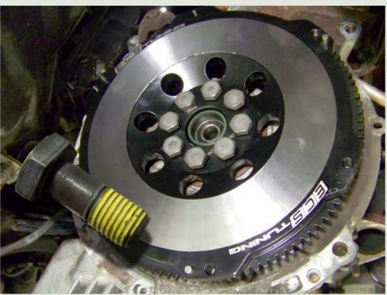
Need to hold the flywheel steady while torquing the bolts? If you don't have the correct flywheel lock, a simple workaround is to loop a length of strong mechanic's wire through one flywheel hole, and them wrap it around a bell housing bolt, threaded in place temporarily. (Multiple strand picture wire is also very strong, and flexible.)
