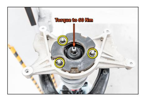
13mm, 15mm Socket & Torque Wrench Step 3:
