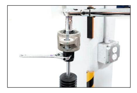
15mm Socket & Torque Wrench Step 2:
