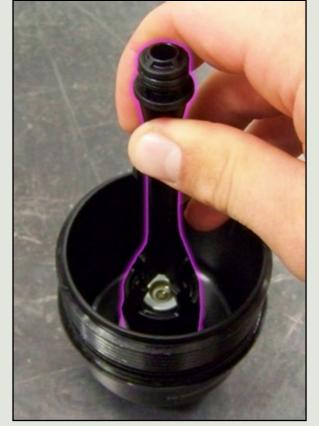
Press the filter post fully onto the base in the housing. Be careful to apply force directly along the axis of the filter post, to ensure it seats correctly and does not break.
