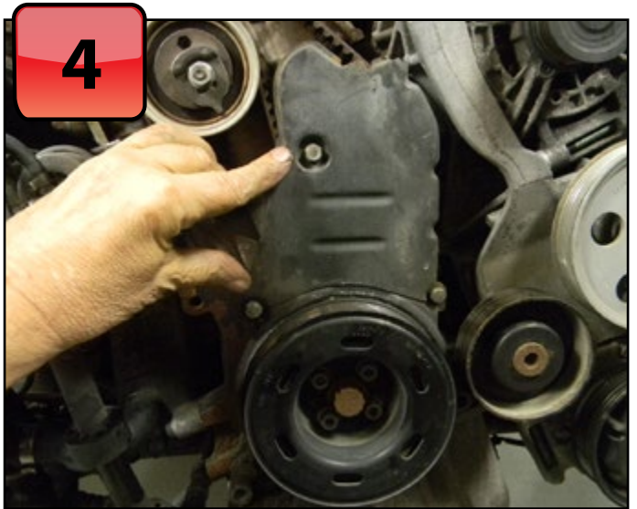
Remove the three middle cover bolts. Remove the middle cover. The bottom cover cannot be removed until we remove the crank pulley.
