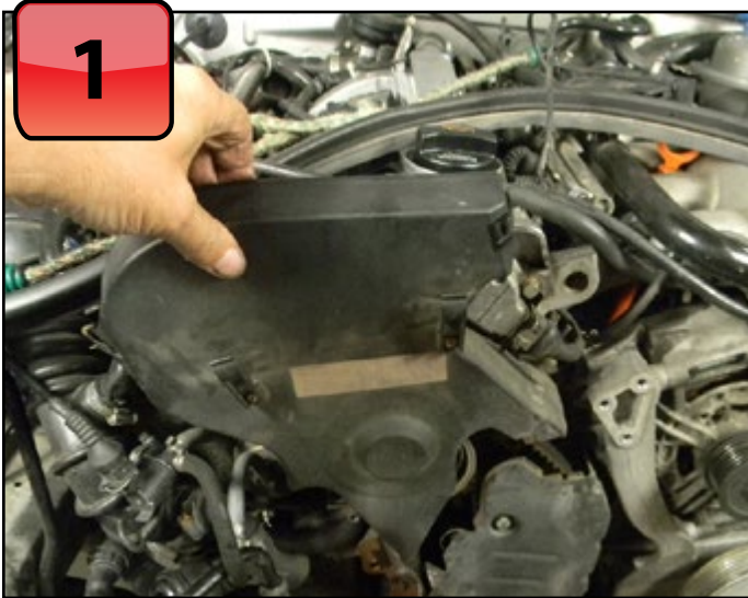
Our sequence starts with the front of the car removed, and the front of the engine exposed. Remove the timing covers. The top cover is held in place by two spring clips; no bolts.
