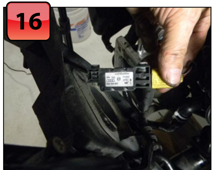
Both crash sensors (one on either side of the radiator support) must be disconnected or unbolted and laid aside.
