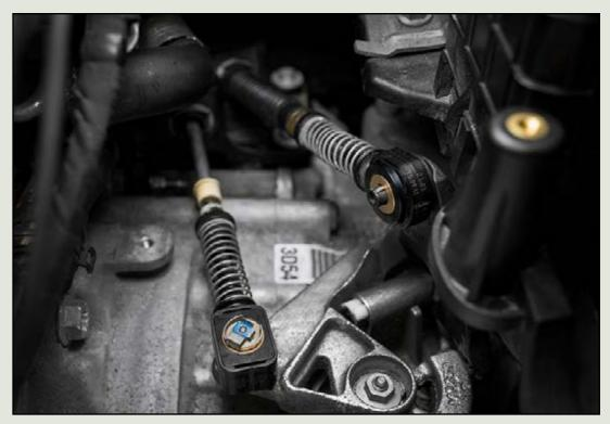
This completes the installation of the ECS Tuning Short Shifter Kit.
