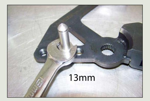
Tighten the shift pin with a 13mm wrench.
