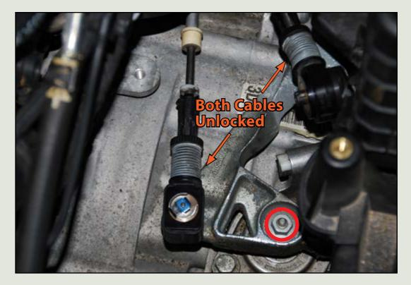
Both cable ends should be unlocked, as shown on the right. Also note here the top of the selector shaft where it is secured to the shift lever (red circle).
