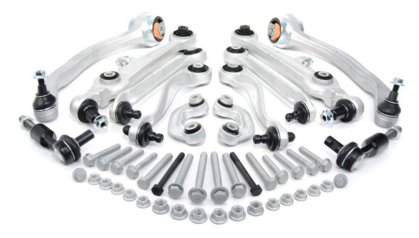
Some kits vary slightly in what they contain, primarily in the inclusion or exclusion of outer tie rod ends or sway bar links. The kit we've decided to install, pictured here, is complete with all eight front suspension links (control arms), two new outer tie rod ends, two sway bar links, and all replacement fasteners.
