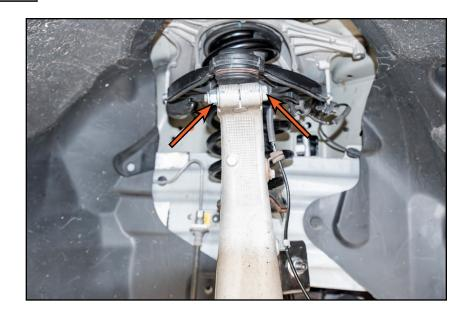
Step 6: 18mm Wrench, T40 Torx Socket & Torque Wrench
