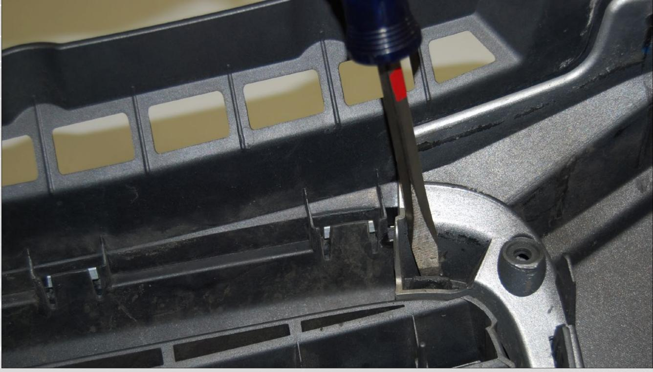
The top corners of the grille have a securing tab that must be carefully released.
