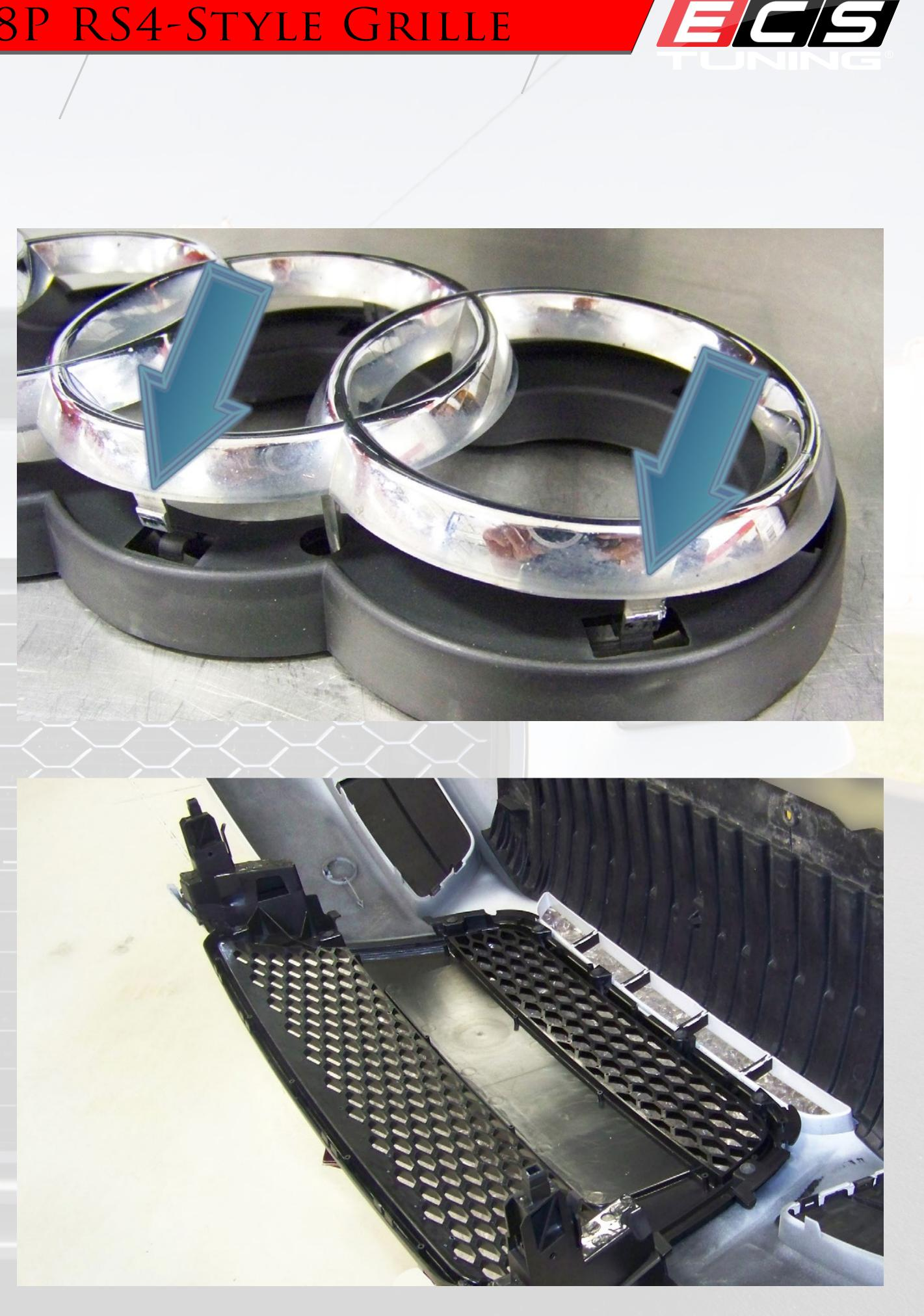
\*The horizontal aluminum bumper support bar, if not modified, will show clearly through the new grille
