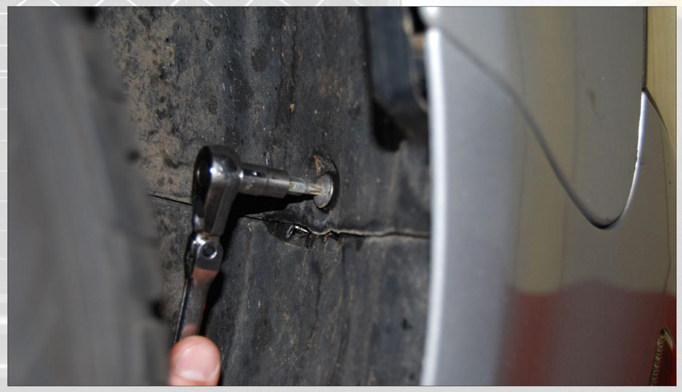
When the fasteners are removed, pull back the flexible fender liner to expose the inside of the bumper cover.
