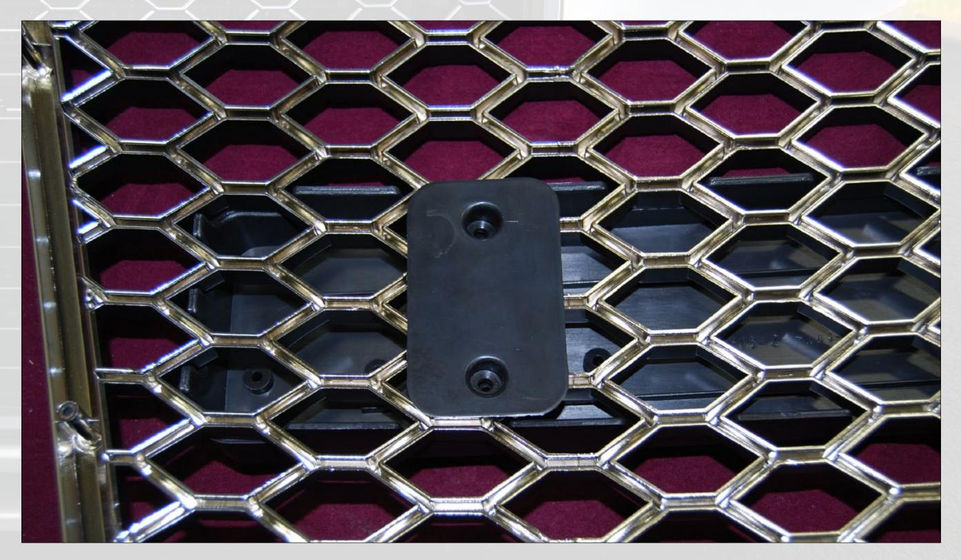
If using the logo bracket, you must remove the original Audi rings from your factory grille. Use a small screwdriver to carefully pry at the tabs until the chrome rings pop free.
