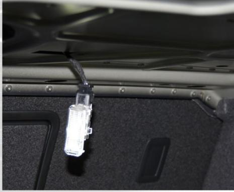
Once your full set of LED's are installed, turn the ignition to the second position and re-inspect each bulb location making sure there is no light flickering.
