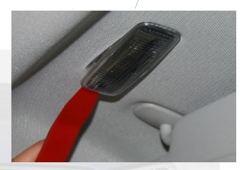
Do not pull with excessive force on the unit; if you are prying at the correct side, the assembly will fall out with little effort.
