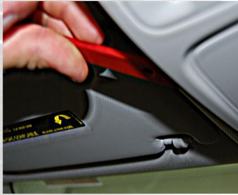
Once you've revealed the bulb housing unit, pry very carefully at the location shown until the front of the bulb housing dislodges partially.
