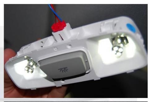
Clip the two halves of the rear dome assembly together, and reinstall the bulb assembly into the vehicle.
