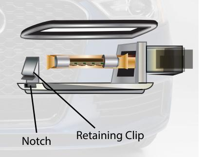
Once the steel backing is revealed, using the non-marring tool or a screwdriver to pry upwards at the location shown, remove the backing.
