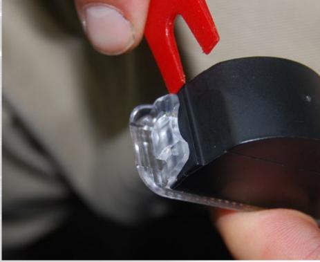
The rear dome assembly consists of two separate units, an outer vanity plate containing two clear lenses, and an inner bulb housing.
