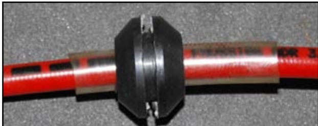
Rubber grommets mounted on transparent polymer sleeves slide back and forth for precise positioning
