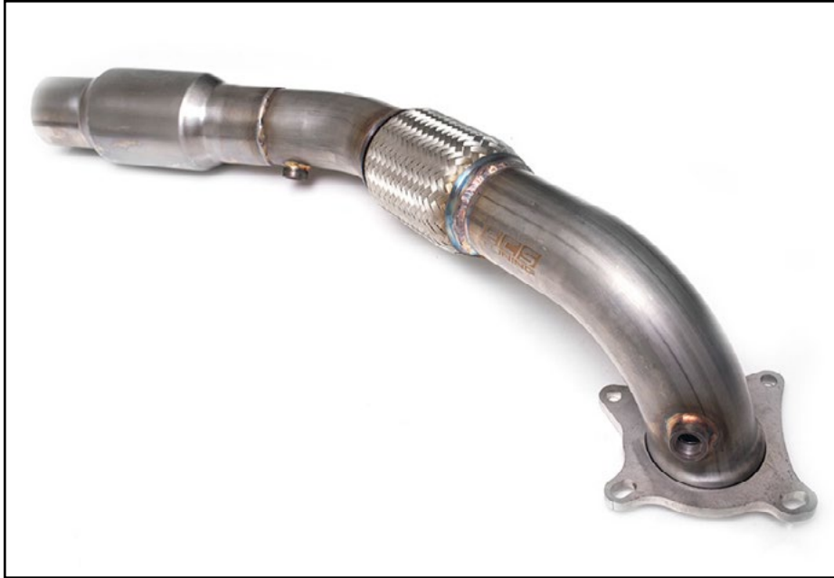
Downpipe w/integrated high flow catalytic converter
