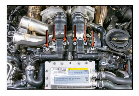
7mm Socket -OR- Flat Head Screwdriver Step 4:
