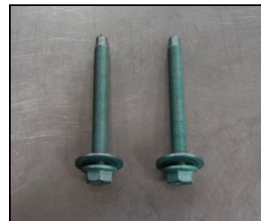
2x Rear Subframe Bolts M12x1.5x110mm
