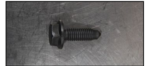
Engine Torque Support Bolt M10x35mm
