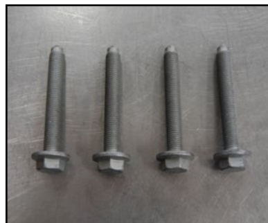
4x Subframe/Control Arm Bolts M12x1.5x90mm
