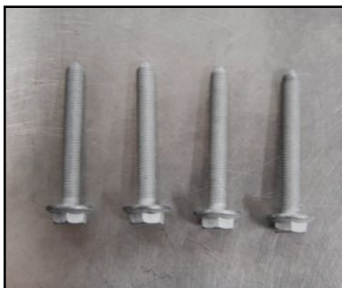
4x Steering Rack Bolts M10x76mm
