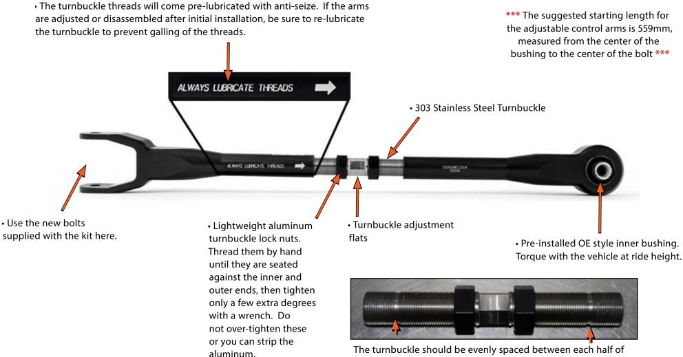
The turnbuckle should be evenly spaced between each half of the control arm. When adjusting, do not extend the control arm halves beyond the grooves (arrows) cut in the turnbuckle threads.
