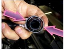
There are several plastic hose connectors used on the engine. Squeeze the circular ring around each connector (arrows) to release the locking tabs and pull the hoses off.
