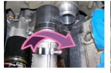
Rotate the clamp heads slightly to the sides so they don't stick up in the air, or they may interfere with the triple pipe when we install it next.
