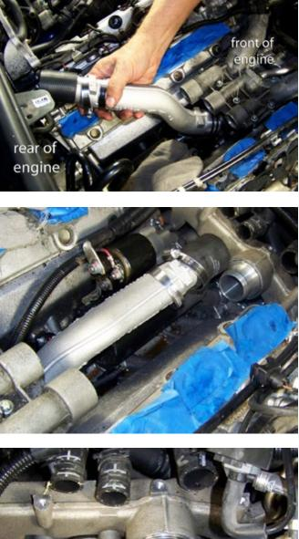
**32**) Rotate the pipe in its bore until its open end aligns with the stub piece. Slide the rubber coupler hose on to the stub piece; position and tighten the hose clamps.
