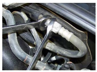
Compress the release tab on the right side fuel line and disconnect it.
