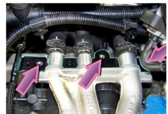
**35**) Install the new breather pipe included in your kit. Snap the elbows over the ports in the engine, and connect the small rubber hose at the rear (arrows). Make sure the lock clips snap in place at the front elbows (lower arrows).
