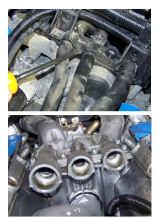
**26)** The only way to remove the large plastic coolant pipe is to cut it in pieces and take it out in chunks. Cut a hole in the top of the pipe (arrow). Suction out any remaining coolant or you will have a mess in the engine valley.
