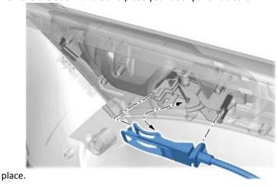
6) Begin to route the White wire through the mirror channel into the interior side of the door. In the bottom near the window motor you will find a 16-pin connector. There are other connectors in this area so make sure you find the 16-pin.
