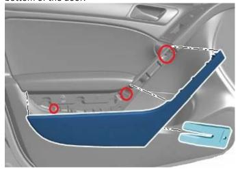
4) Once the screws are removed, tug the panel separating it from the door. There are several clips attaching the panel to the door.
