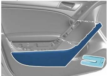
3) There are 4 Torx screws total holding the door panel on. (3) Behind the panel and (1) at the very bottom of the door.
