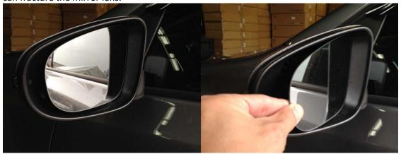
2) Once the lens is removed, remove the two T10 Torx screws to remove the frame from the housing.
