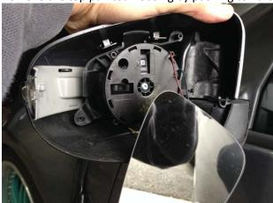
5) To remove the bottom housing, squeeze the circled clip and drop downward to remove. Unplug the connector going to the turn signal and replace with new lower.
