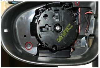
3) There are two clips that lock the housing together. Disengage those and the housing frame will separate pulling forward.
