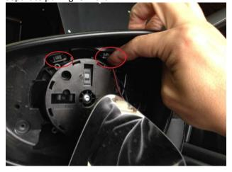
4) Remove the top painted housing by pushing towards front of vehicle.
