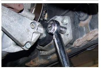
This completes the installation of the heavy duty polyurethane snub mount bumper.
