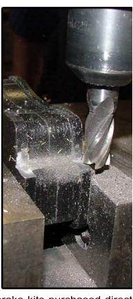
As of February 15th 2004, all MKIV Volkswagen Stage 2version2 big brake kits purchased direct from ECS Tuning require minor pad modification. Kits purchased prior should continue to us unmodified pads. This change is due in fact that ECS no longer modifies the caliper guide pins allow the pads to sit close to the rotational center of the rotor.
