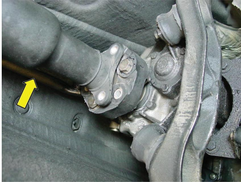
Begin by removing the shifter linkage shown in the photo. On both ends there is a clip that can be pushed upwards to encourage removal. Once the clip is removed pull the rod from the socket.
