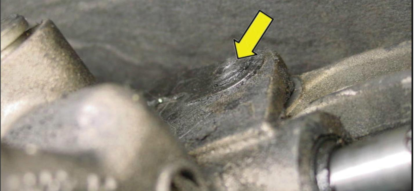
This clip can be very difficult to remove. In E90+ series the clip was redesigned for easier removal.
