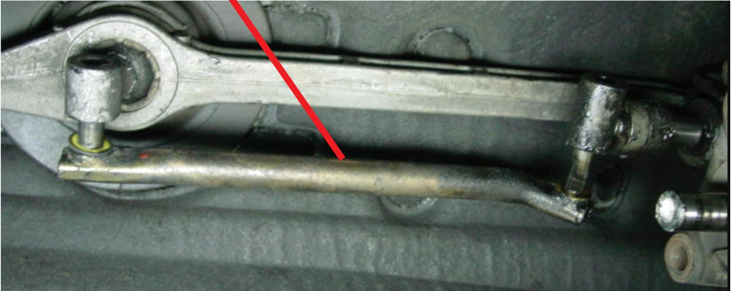
The driveshaft was removed for visualization purposes. This shifter can be installed with the driveshaft in place. This is the orientation of the shifter assembly attached to the transmission
