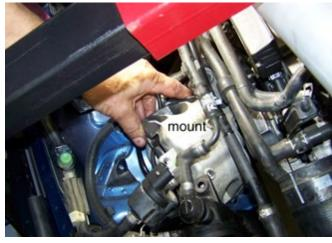
Step 13 Remove the top bolt holding the lower engine mount to the engine block.
