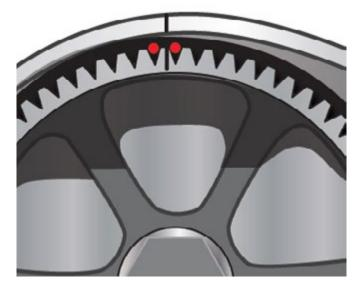
In addition to the timing marks, add a separate arrow indicating direction of rotation.
