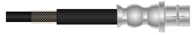
**Assembly:** Hoses are cut to length, then metal fittings are inserted and crimped onto the ends of the hose. The lines are pressure tested to ensure they can handle the high pressures of the braking system before being packaged.
