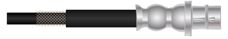
**Assembly:** Hoses are cut to length, then metal fittings are inserted and crimped onto the ends of the hose. The lines are pressure tested to ensure they can handle the high pressures of the braking system before being packaged.
