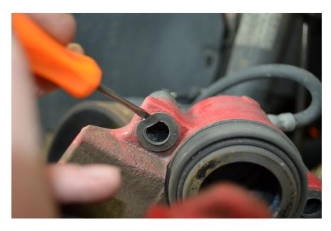
Be sure the hole for the bushings are clean and free of corrosion and debris. You can use some high grit sandpaper or a scotch brite pad to clean it out. Clean the outer surface and the bushing bore.
