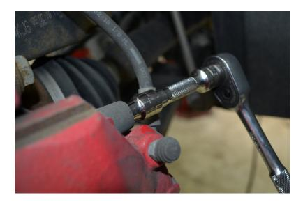
Slide the caliper off the carrier and secure it on top of the rotor or with a bungee cord as to not put excessive tension on the hydraulic line.
