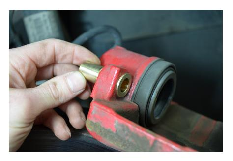
Do NOT use a hammer or excessive force to install the bushings. If for any reason they do not fit or are hard to go in, please give us a call. They should slide in very easy.
