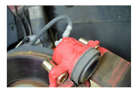
Install the pads and reinstall the caliper back onto the caliper bracket.
