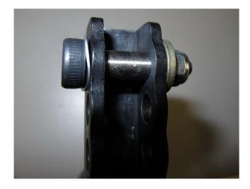
Note: You can try the other mounting holes and even try removing the spring all together if you'd like in the future. Remember if you remove the spring all together, you should remove the upper spring mount as well as it can become pinned against the arm when not held in place with the springs.
