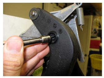
The plastic pivot push pin will be replaced by the UCP clutch master shoulder bolt and nut.
