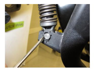
Remove only the spring locator on the arm itself – leave the upper pivot barrel and c-clip in place.
