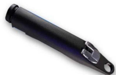
There are many cheap testers on the market, some costing less than cheesburger. We prefer a refractometer for accurate measurements. This precision measurement device will last a lifetime with careful use. It measures freeze protection of ethylene and propylene glycol coolants, and the specific gravity of battery acid, as an added bonus.
